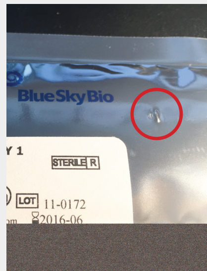
50 | Sterile packaging compromised by a sharp-edged cover screw (BlueSkyBio).
